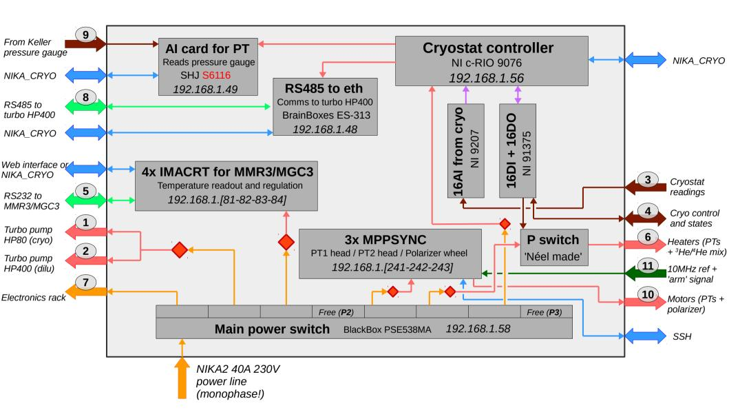
**NOTES**: - all Ethernet connections actually pass through a switch, so that only 1 Ethernet cable connects this box to the rest of the NIKA network! - the numbers are used to show where each of the outputs is located on the main 'interface panel' (see page 4!)
