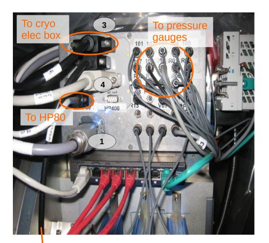
To pneumatic attenuators for cryostat inclination control
