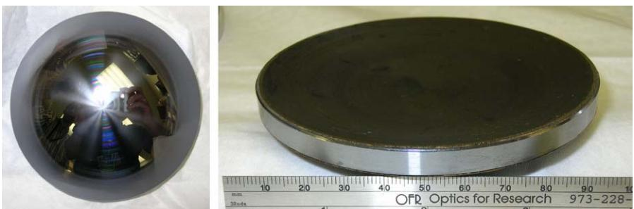
**Fig. 4** (Color online) The 10 cm silicon lens used in GISMO before (*left*) and after (*right*) the AR coating which applied at Princeton University
