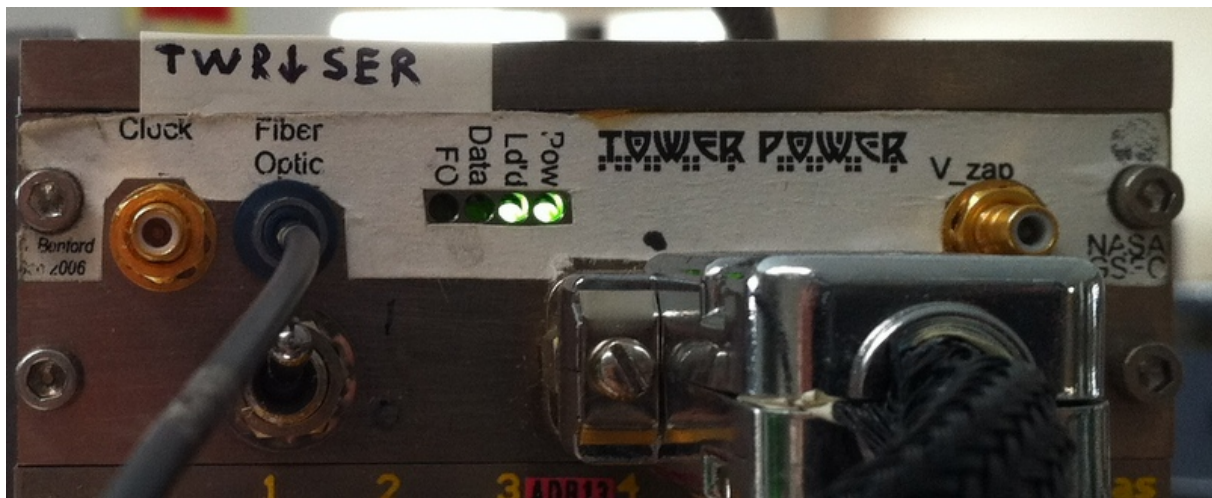
Top part of the Tower showing tower serial fiber ("TWR SER") connection (from gismo-detector), tower power connection, and nominal light indicators (the "Data" light will flash when data is sent [e.g., during startup or tuning])
